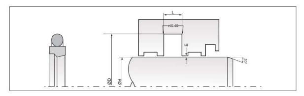
d: 55, D: 65.7, L: 4.2 MOC: Sealing Ring: Bronze filled PTFE O Ring: NBR / FKM 70/75 shore A Qty: 1No
