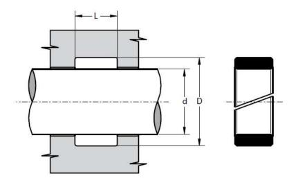
D: 55, d: 61, L: 25 MOC: Acetal resin with glass fibre (BEARITE) Qty: 1No
