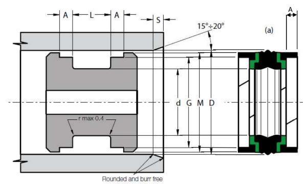
D: 80, d: 60, L: 22.4, A: 6.35, G: 74.15, M: 78.3 MOC: Seal ring: Nitril Rubber (RUBSEAL 75) NBR with Hardness: 75 °ShA Anti-extrusion rings: Thermoplastic polyester resin (SEALITE 63) with Hardness: 63 °ShD Guide rings: Acetal resin with glass fibre (BEARITE) Qty: 1set
